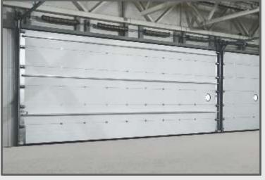
TLP - ULTRA THERMO size limitations: maximum width 12 meters. max height 8 meters, max 70 m<sup>2</sup>.
